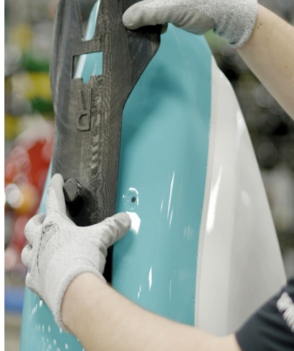
A soft-touch, flexible assembly tool made from TPU 92A elastomer locates a badge on the motorcycle tank without marring the painted surface.
