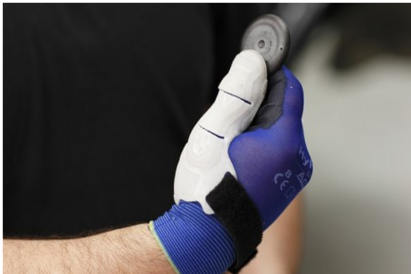
The white 3D printed thumb tool provides leverage to reduce fatigue and prevent overuse injury when inserting these plastic plugs.
