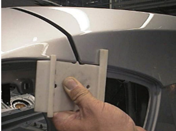
A worker inspects the fit on this auto assembly using a 3D printed check gauge.
