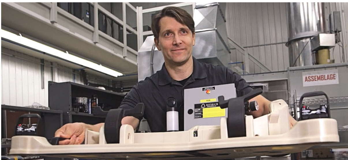
3D printing this automotive door seal jig resulted in an 80% weight reduction and a decrease in task cycle time.
