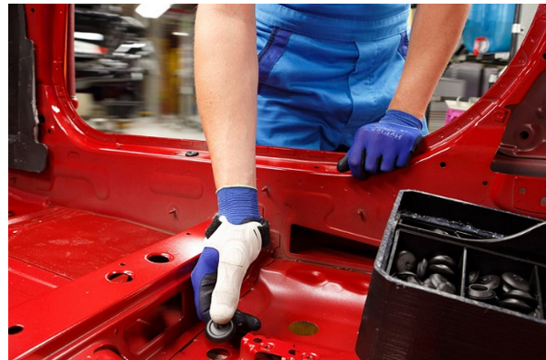
The white 3D printed thumb tool provides leverage to reduce fatigue and prevent overuse injury when inserting these plastic plugs.
