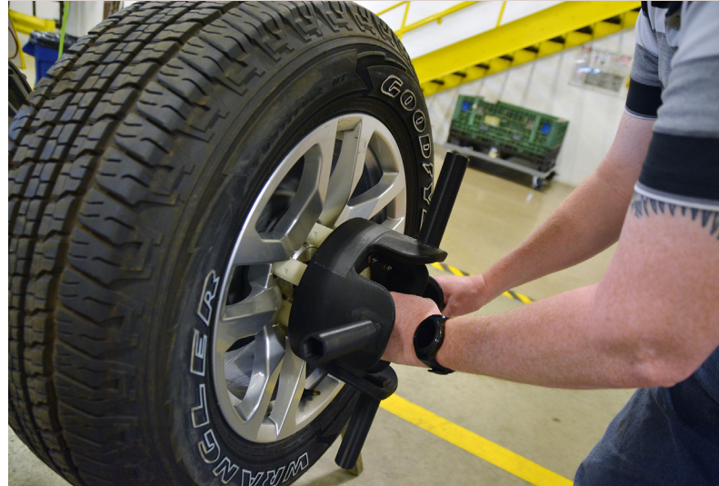
This 3D printed assembly tool provides a lighter, faster means of installing wheel lug nuts.
