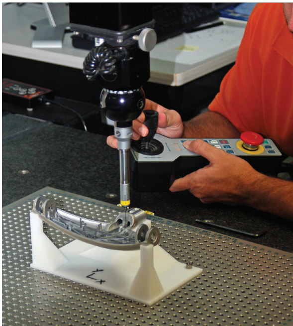
This CMM inspection fixture was created in a fraction of the time it would take to manufacture metal tooling.
