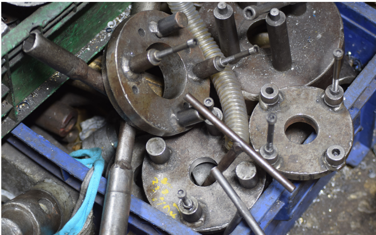
3D printed tools can replace typical metal, multi-part, welded assembly jigs like this.
