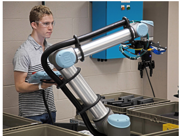
Lighter 3D printed end-of-arm tools reduce the load on robotic arms and are typically faster and less costly to make than their metal counterparts.
