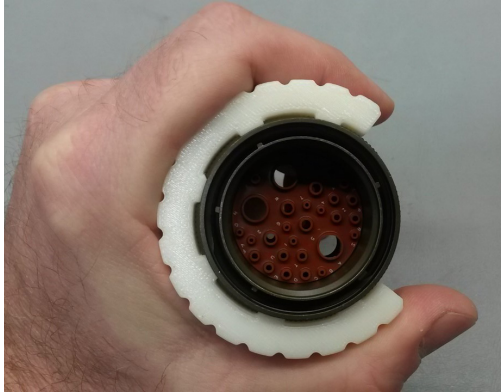
This 3D printed gripper gives workers a more comfortable way to grip the connector, reducing fatigue.
