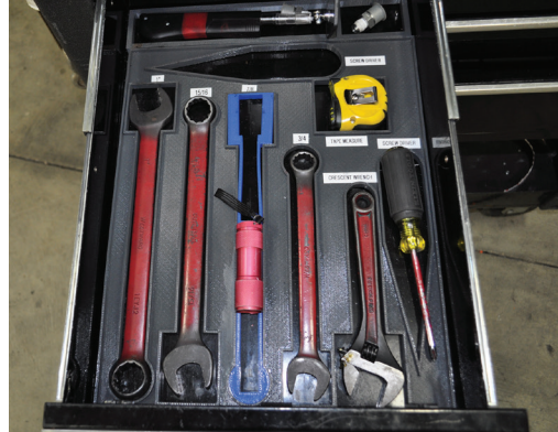
The design freedom of additive manufacturing makes it easy to create custom tool holders and sorting trays.
